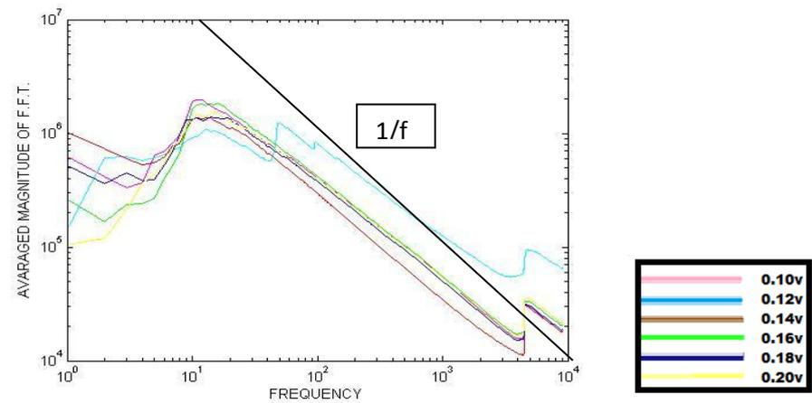
Fig 3.6 for Different Drain Voltages at  $V_g = 3.65V$  1/f Noise in the MOSFET IRF 340
