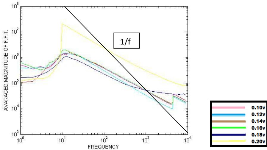
Fig 3.5 for Different Drain Voltages at  $V_g = 3.25V$  1/f Noise in the MOSFET IRF 340
