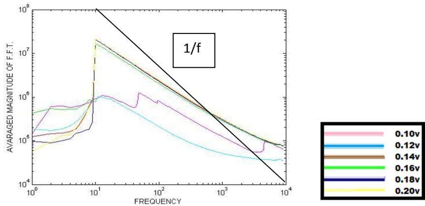
Fig 3.3 for Different Drain Voltages at  $V_g = 3.50V$  1/f Noise in the MOSFET IRF 440
