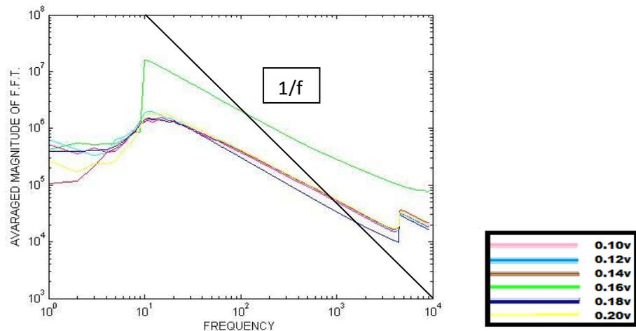
Fig 3.4 for Different Drain Voltages at  $V_g = 3.95V$  1/f Noise in the MOSFET IRF 440
