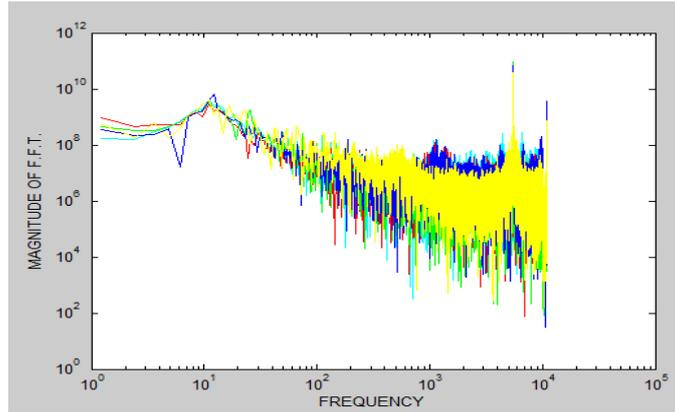
Fig. 2 FFT Amplitude of IRF 640 for Different Drain Voltages
