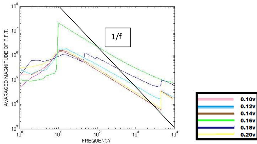
Fig 3.2 for Different Drain Voltages at  $V_g = 3.92V$  1/f Noise in the MOSFET IRF 640
